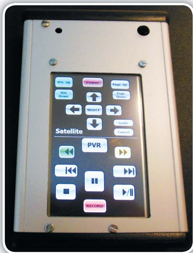
Photo 1: This is a touch-screen multi-function IR remote control I built a while back, using 4D Systems uLCD-43PT intelligent TFT touchscreen module. I am now designing a similar device using the much less expensive EVE display modules.
