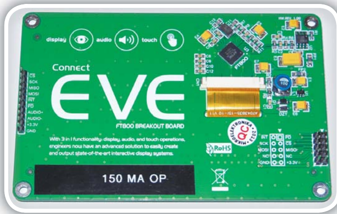
Photo 2: This is the control PCB side of the Connect-EVE 4.3" display module. Note that it contains both a 10 pin interface and a 2X5 header, with all necessary signals available on both. The "150 MA OP" label is one that I added to remind me that the module draws 150 milliamp when operating, which is important since I am using it in battery-powered projects.
